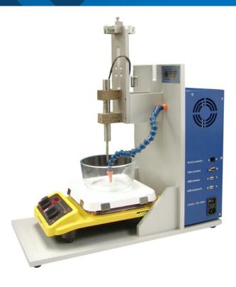
AVID Innovation's BFR200 Bend & Free Recovery tester is a compact, fully integrated, user-friendly test system for measuring transformation temperatures of Nitinol-based components and devices.
